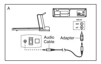
B. Plug one end of the audio cable into the jack on the front of the Incline Trainer near the power cord. Plug the other end of the cable into the included adapter. Plug the adapter into an RCA Y-adapter (available at electronics stores). Next, remove the wire that is currently plugged into the AUDIO OUT jack on your VCR and plug the wire into the unused side of the RCA Y-adapter. Plug the RCA Y-adapter into the AUDIO OUT jack on your VCR.
